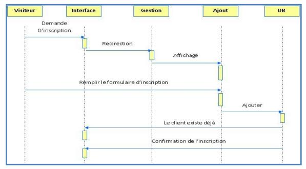
Figure 9: Registration sequence diagram - The
